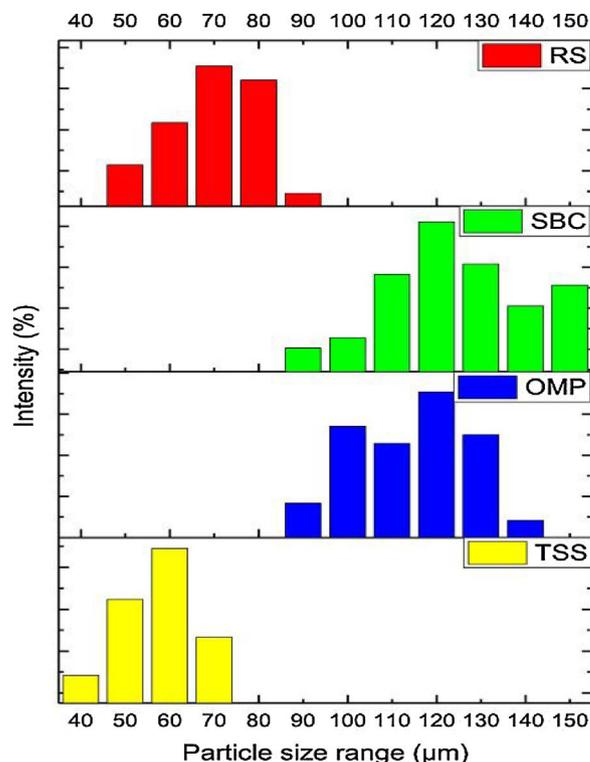
Fig. 4. Particle size distribution of Bio-thermoplastic polysaccharides extracted from agro industrial wastes.
