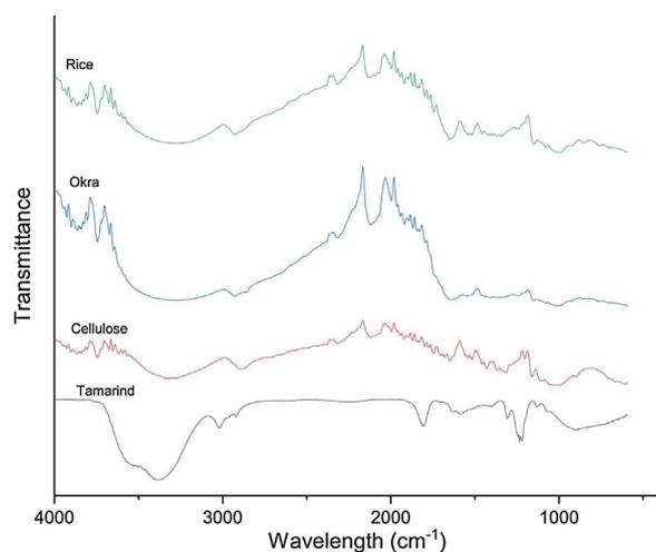
Fig. 3. Fourier transform infrared spectroscopic bands of isolated Bio-thermoplastic polysaccharides.
