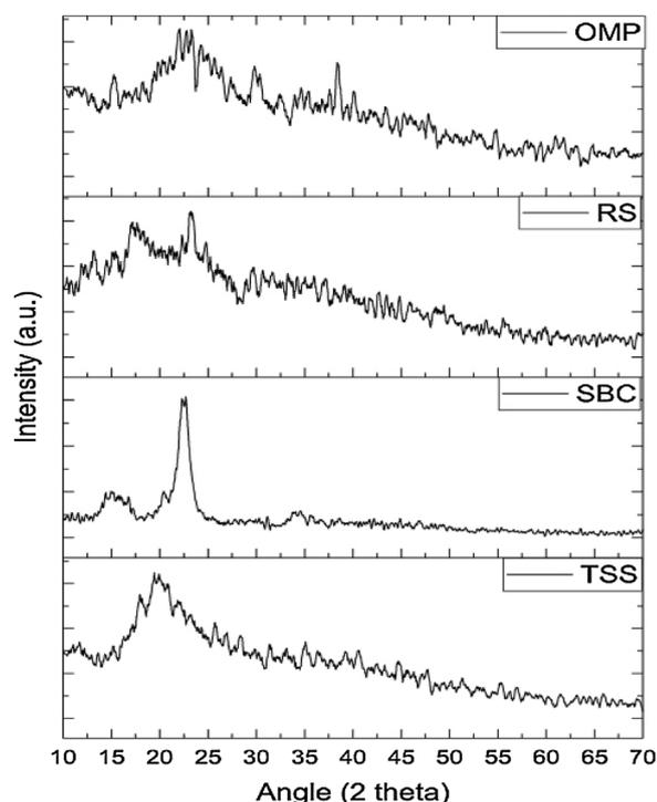
Fig. 2. X-Ray diffractogram pattern of isolated Bio-thermoplastic polysaccharides.
