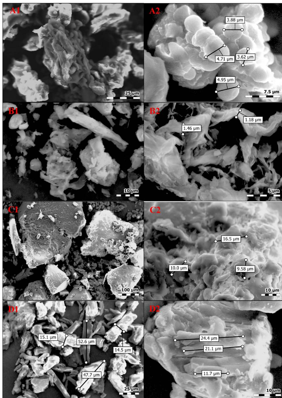
Fig. 5. Surface morphology of extracted polysaccharides [Tamarind seed starch [A], Okra mucilage [B], Rice bran starch [C], Sugarcane bagasse cellulose [D]].
