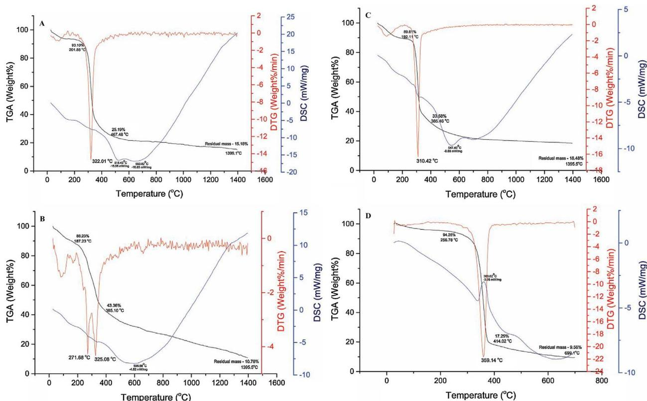
Fig. 1. TG-DSC analysis results of extracted Bio-thermoplastic polysaccharides [Tamarind seed starch [A], Okra mucilage [B], Rice bran starch [C], Sugarcane bagasse cellulose [D]].
